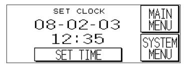
This screen allows the user to set the 7-day timer which can be programmed for daily or weekly (over midnight) on/off operation. An internal battery backup holds the settings in memory when the dryer is de-energized.
